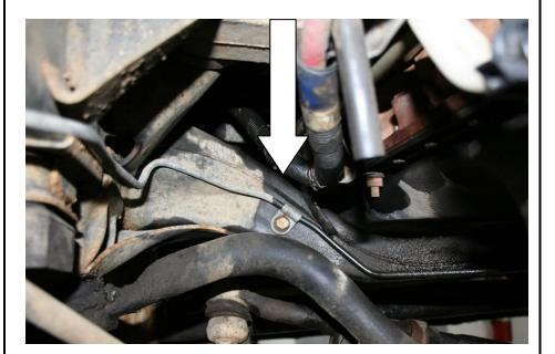
Insert tapered insert (#1302042Z) into the driver's side track bar mounting hole.
