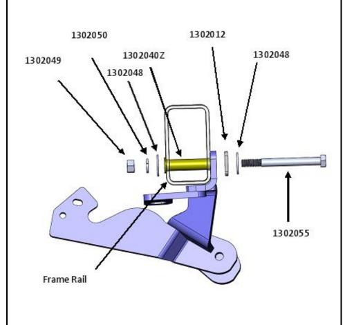
With the retrofit bracket, loosely in place, we can now focus on the rear of the cross member.
