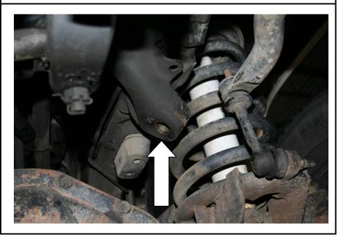
Clean the outside frame rail where the retrofit bracket will mount.
