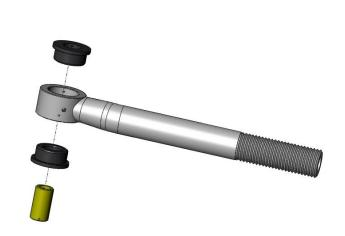
Use the remainder of the supplied grease and rub it all around each half of the bushing (ID and OD). Once fully lubed press the each half of the bushing into the track bar ends. Finally lube the steel sleeve and press into the bushings.
