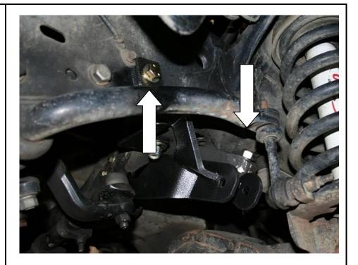
\* You will only need to use the second 1302044 washer if the weld line is very large on the driver's side factory track bar mounting face.
