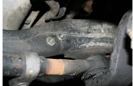
Now using the remaining ½" x 5" bolt to secure the last bracket point.
