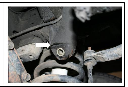
You can now insert the ½" x 4.5" (#1302055) bolt and hardware securing the retrofit bracket to side of the frame.
