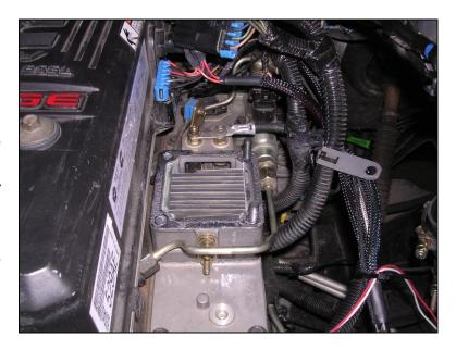
With the jam nut supplied you will need to double nut each stud and torque the stud down in place to 3 lbs-ft. You must make sure that the threads are fully seated in place. Once it has been torqued, you can remove the two nuts.
