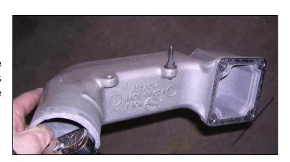
You will now need to scrape off any left-over gasket material that resides on the intake heater.
