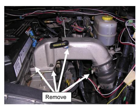
On the rear of the intake you will notice a wiring harness bolted to the intake. You will need to remove the nut and washer that secure the wiring harness to the intake.
