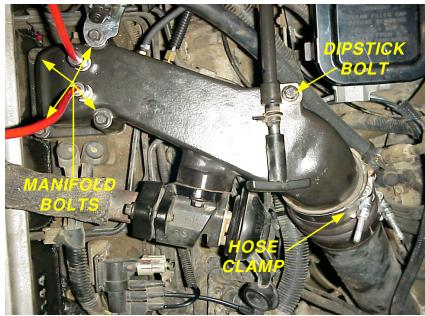
Figure 2 - Dodge 12V Intake Manifold
