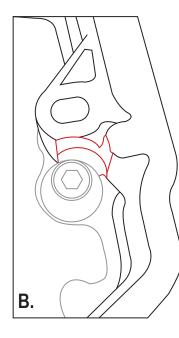
B. Remove material as necessary to allow clearance for stud, nut and washer. Finish machine work should allow easy removal and installation of the head stud.
