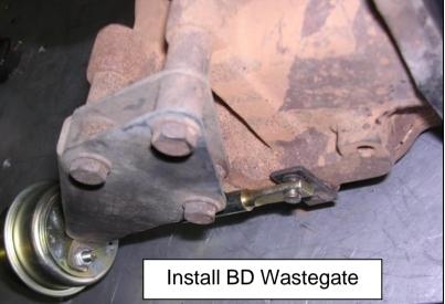
the rod end forward. Align the wastegate arm hole with the BD rod end and insert and lock into place with the supplied cir clip. Once the clip is in place you can then tighten the mounting nuts.
