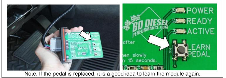
14. Snap cover back on module and mount the module below the dashboard or in the engine bay for 1998.5-2004 Dodge trucks.
