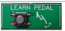
will allow the module to learn your specific accelerator pedal sensor output. Make sure the pedal travel is not impeded by a floor mat. Once complete, the LED indicators will go back to their normal function. Turn the ignition switch back off. The module is now learned to your APP sensor and will retain this in its memory.
