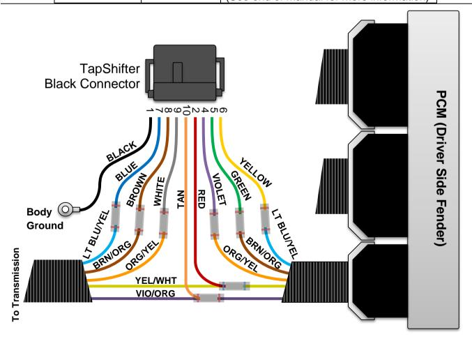
Use electrical tape to loom up the wires and slip the original wire loom over the connections. Leave the black wire with ring terminal from the BD kit to hang outside of the harness. This will be connected to a body ground.
