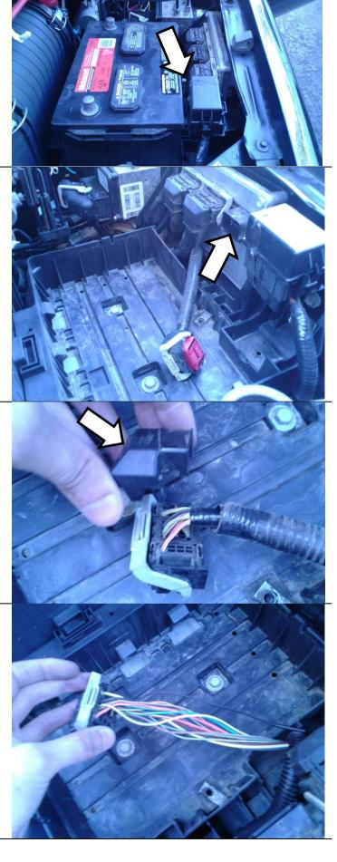
Make the wire connections as shown in the following diagrams using the supplied heat shrink butt connectors.
