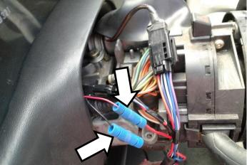
The shift lever wiring must be carefully secured to reduce chances of failure due to pinching or chafing.
