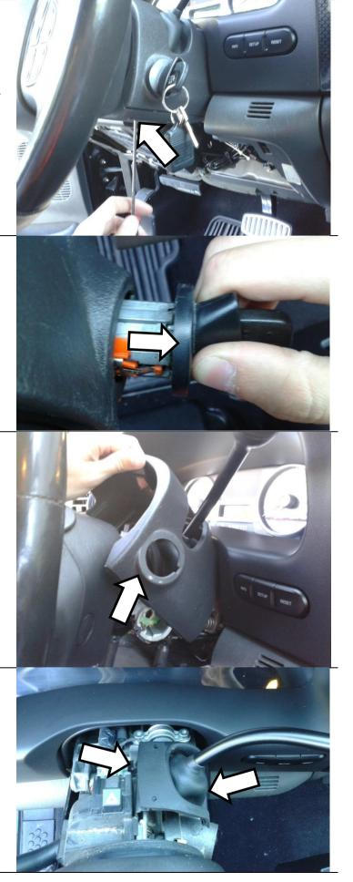
Using a punch and a hammer, drive the "press in pin" out of the shifter assembly. This will allow the shifter handle to be removed from the vehicle.
