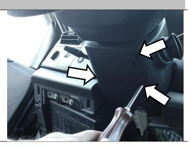
To remove the upper cover the ignition lock cylinder must be removed. Insert a long pick or similar tool into the hole beneath the switch and push upwards while rotating the key to the on position.
