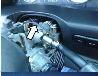
Move the shift lever through the gears and make sure the wire does not get pinched.
