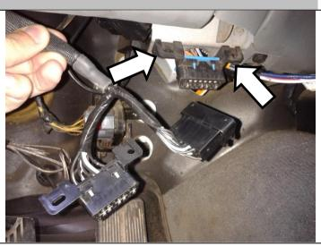
The OBD connection can be left in place if simply changing tune "power levels" on the fly, but if left connected during an ECM/PCM/FICM flash program/update it will cause the connection to be interrupted. If this is a concern, the original OBD connector can be left in place and the TapShifter wiring tied out of the way. This way it will be obvious to others that there is a device connected to the OBD port.
