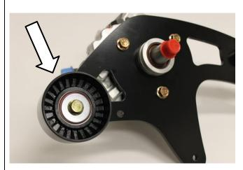
24. Install bracket and pump assembly onto the front of the engine. Using the OEM bolts from the cooling fan pulley hub. Using a 13mm socket, snug the bolts hand tight at this point.
