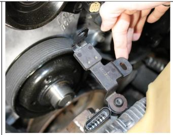
44. Stack the 1500726 bracket on top of the OEM fan clutch bracket, and insert OEM bolt through both.
