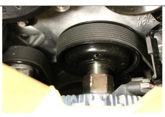
46. Torque fan bracket bolt to 18 ft-lbs, using a 13mm socket and reconnect fan clutch connector.
