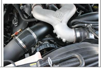
69. Prime fuel system several times using the filter pump, or lift pump and start engine. Check for leaks.
