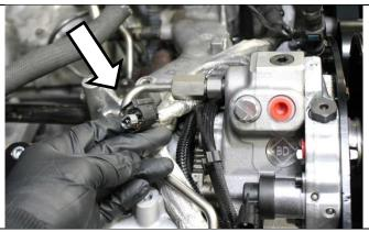
34. Plug-in supplied wiring harness 1500722 into OEM CP4 connector, and CP3 as shown.
