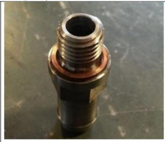
38. Install 1502040 HiFlow pressure feed fitting sealing washer, and torque to 6 ft-lbs.
