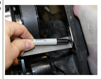
50. Drill two(2) 6mm(.236in) diameter holes on marks made in previous step.
