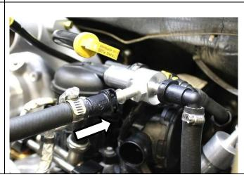
64. Trim to length and push hose over feed fitting on CP3 pump. Secure with 1452821 gear clamp.
