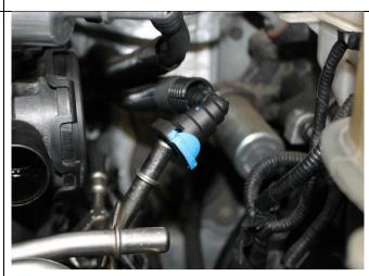
60. Install second quick-disconnect adapter onto return outlet (arrow 2). Apply FT-0606434 Loctite to 1500720 retaining collar (arrow 1), and slide over outlet, behind shoulder, and thread into adapter. Torque to 10 ft-lbs.
