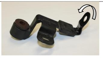
43. Re-install OEM fan connector bracket to fan clutch. Leave connector off of bracket.
