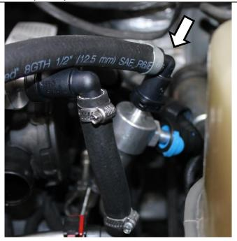
67. Trim fuel tube to length, and secure with 1500387 spring clamp.
