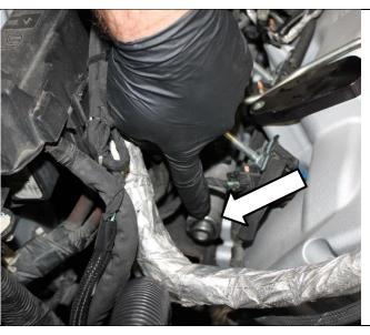
31. Install supplied fuel rail fitting 1500704, into previously plugged port (front end of passenger side fuel rail). Using a 22mm socket, torque to 75 ft-lbs.
