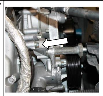
12. Remove both idler pulleys using a 15mm socket. These will be relocated to CP3 bracket, once installed.
