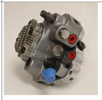
22. Mount CP3 pump to CP3 bracket 1500714. Use three(3) supplied 1453934 Bolts, six(6) 1401556 Washers, and three(3) FT-1190681 Nuts. Torque fasteners to 20 ft-lbs using a 13mm socket, and 13mm wrench.
