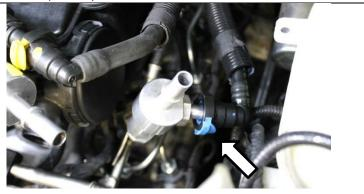
62. Insert 1500723 quick-disconnect fitting into end of supplied 1/2in fuel hose, and secure with 1452821 gear clamp.
