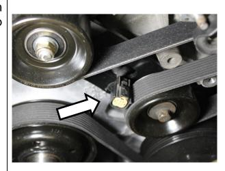
42. Before installing cooling fan assembly it may be helpful to adjust OEM fan connector bracket by bending the metal tab slightly forward as shown. This is done to accommodate the installed CP3 bracket thickness.
