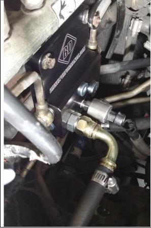
19. The connections for the factory WIF sensor and fuel heater will now be exposed. It is highly recommended that a WIF extension harness be installed into the factory connector to allow the use of an auxiliary WIF sensor.
