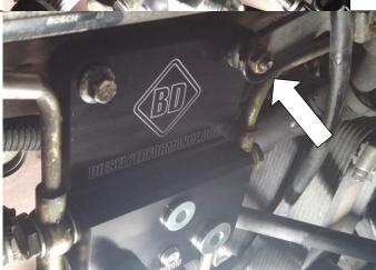
17. If running the fuel feed through the distribution block, attach the supplied swept -8 JIC to a ½" fuel hose (not supplied), and connect the hoses to their respective fittings.
