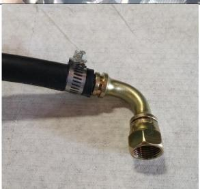
18. Ensure all fittings are tight, and hoses are zip tied away from any hot or moving parts in the engine bay.
