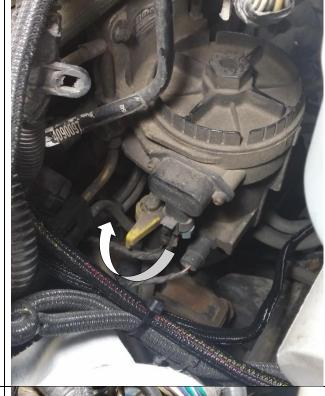
3. Remove dipstick mounting nut from the fuel bowl mounting bolt using a 10mm socket. (5.9L engine only)
