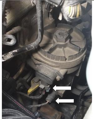
5. Remove bolt holding the return line to the back the of fuel bowl using a 10mm Socket.
