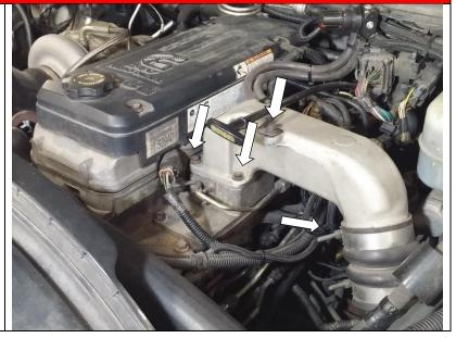
Place a pan or bucket below the fuel bowl and drain as much fuel out as possible by turning the drain valve. This will help reduce fuel spill when the fuel lines are disconnected.
