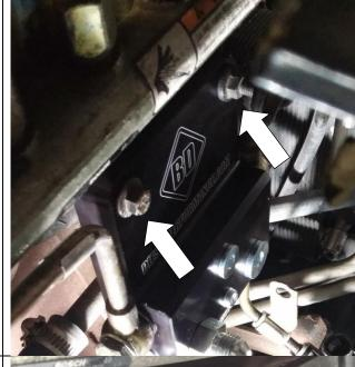
16. Re-install dipstick onto stud, and tighten nut to **6.7 Ft-Lbs**. (5.9L Engines only)
