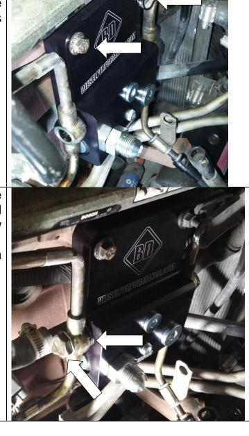
15. Tighten the two bolts holding the fuel distribution block to the cylinder head using a 10mm socket to **24 Ft-lbs**.
