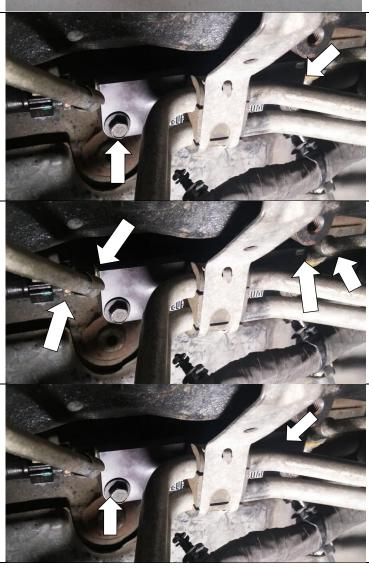
18. Using the supplied insulated loop clamp, and bolt. Secure the starter cables to the top of the motor mount.
