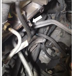
Remove the three (3) screws holding the bracket to the engine using a 10mm socket. Remove bracket from engine.
