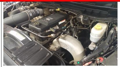
Place a pan or bucket below the fuel bowl and drain as much fuel out as possible by turning the drain valve. This will help reduce fuel spill when the fuel lines are disconnected.
