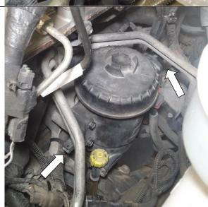
4. Disconnect the factory fuel quick connects from the fuel bowl, if still in use.(Fuel bowl shown removed for clarity)
