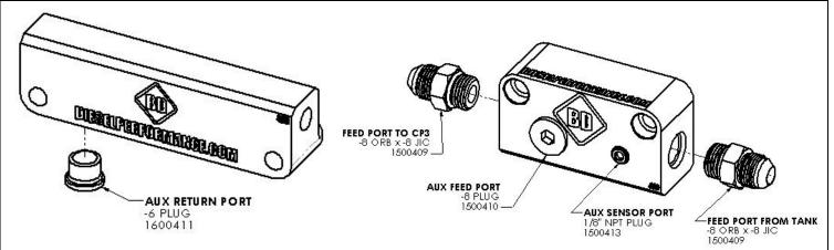
12. Shown is how a typical install could look like with the fuel feed block.
