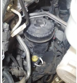
3. Disconnect the fuel heater and WIF sensor connectors.
