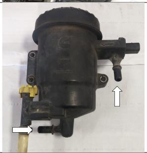
5. Remove the three (3) bolts holding the fuel bowl and filter assembly using a 10mm socket, and remove the bowl from the engine bay.
