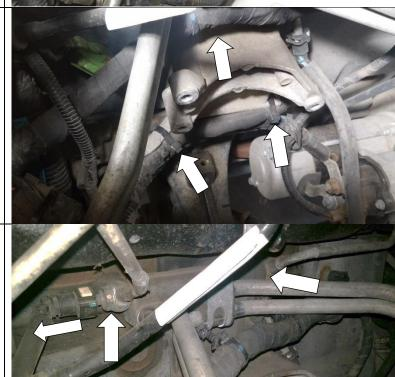
7. Remove the return quick-connect and remove banjo bolts from both sides of the fuel return bracket with a 17mm socket. Set these aside, as they will be re-used later for install.
