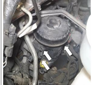
6. Cut zip-ties holding battery cables, and pull the upper wiring harness off the fuel bowl bracket.
