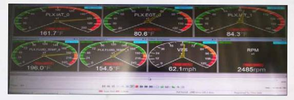
Air intake temperatures (AIT) were recorded from the inlet and outlet of both intercoolers using PLX K-type thermocouples. Boost pressure was also tested to ensure that no dramatic pressure drop occurs when installing the larger Mishimoto intercooler. Mechanical gauges were used because of the high boost levels.
