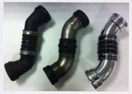
decreases. The cold-side intercooler pipe was designed to be 3.5" with smoother bends, allowing for greater airflow compared to the plastic stock unit.
